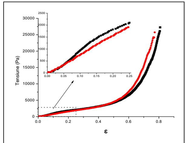
Figure 2. Compression curves for the 5% apricot supplemented bread (■sample 1; ● – sample 2)
