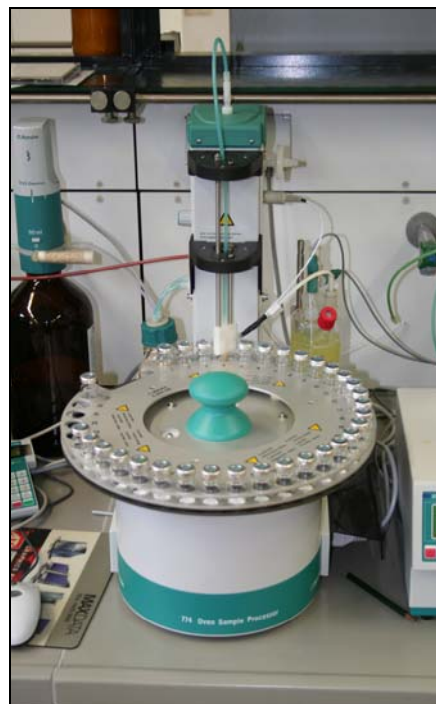
Figure 6: Sample rack of the automated Karl Fischer titration with heating oven.
