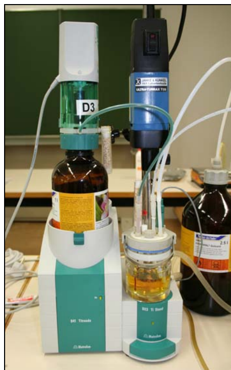
Figure 3: Karl Fischer titrator with a heatable titration vessel.
