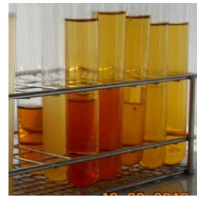
Figure 5. Multiple tube method-positive reaction Streptococcus fecalis (shifting of the medium to yellow/turbidity)
