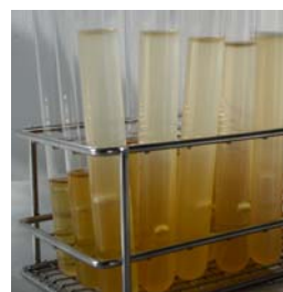
Figure 1. Multiple tube method-positive reaction for coliform bacteria (turbidity/gas production in Durham tubes)
