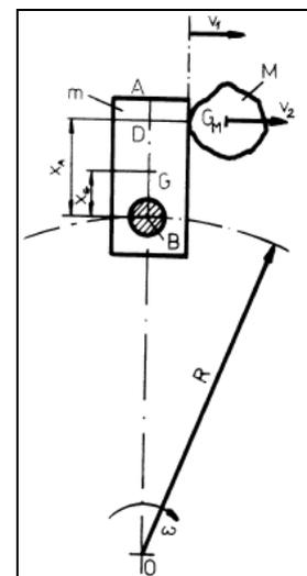
Figure. 1 The percussion between the hammer and the material particle
