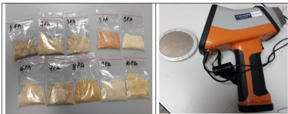
Figure 1. The pasta samples and the XRF analyzer device
