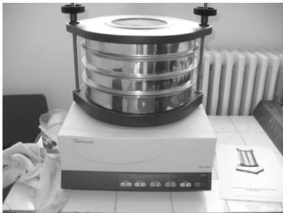
Figure 3. Sieving machine AS300
