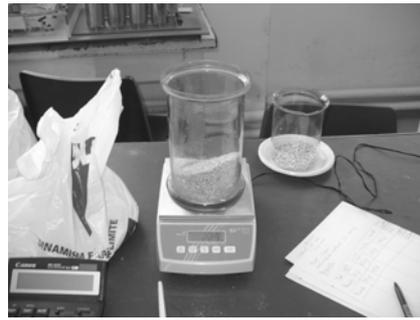
Figure 6. Weighing one mix sample
