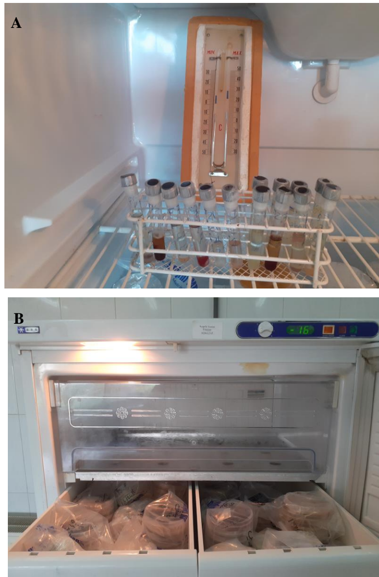
Figure 1. Stocks and Preserved cultures of Fusarium spp. and Cochliobolus sativus in (A) a standard refrigerator at 4°C, and in (B) a standard mechanical freezer at -16°C
