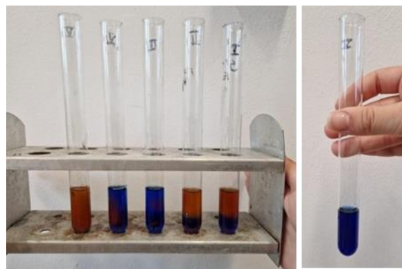
Figure 3. Variation of glucose content in the analyzed samples, highlighted with the Fehling test.
