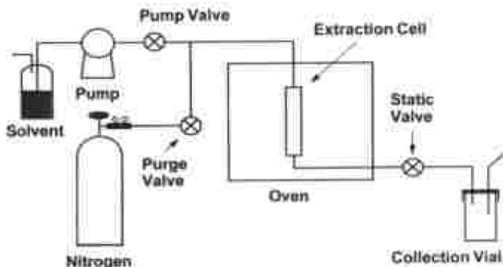
**Fig 3.** Scheme of Pressurized Fluid Extraction (PFE)
