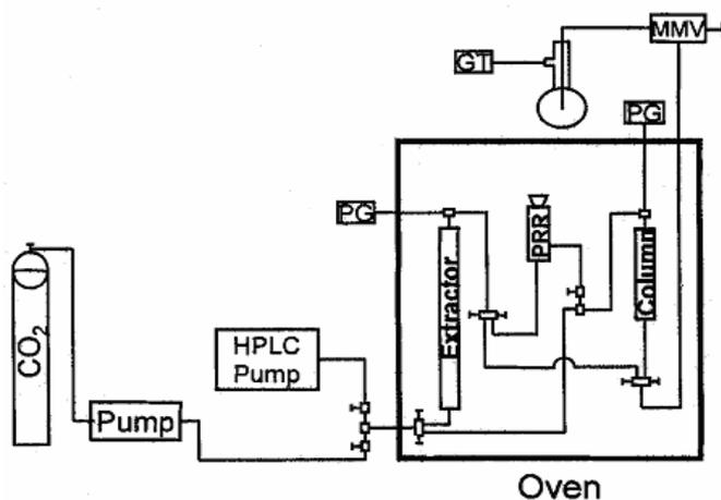
**Fig. 4.** Schematic of supercritical fluid extraction /supercritical fluid Chromatography (SFE / SFC) processing system. Pressure gauge (PG); gas totalizer (GT); micrometering valve (MMV); pressure-reducing regulator (PRR).
