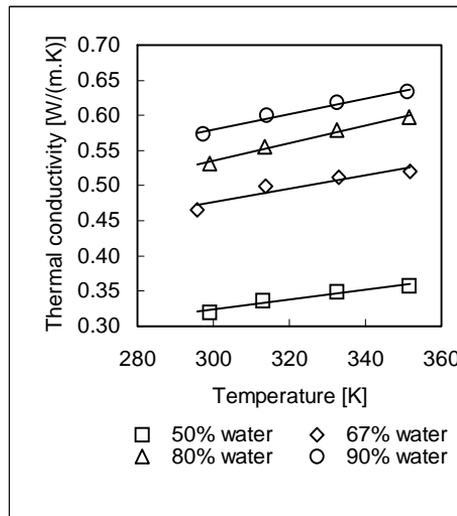
**Fig. 2.** Concentrated milk thermal conductivity versus temperature at different water contents
