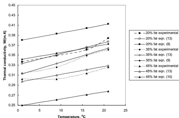
**Fig. 3.** Thermal conductivity of cream versus temperature, at different values of the fat content
