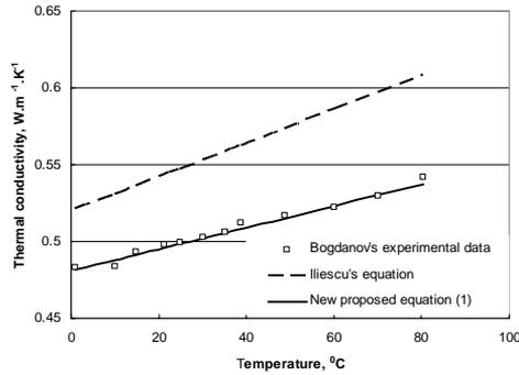
**Fig. 1.** Thermal conductivity of whole milk (3.2% fat) versus temperature
