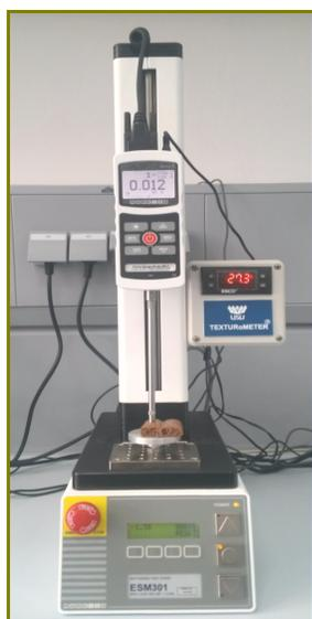
Figure 1. Texturometer Mark-10-ESM301 [4],[5]
