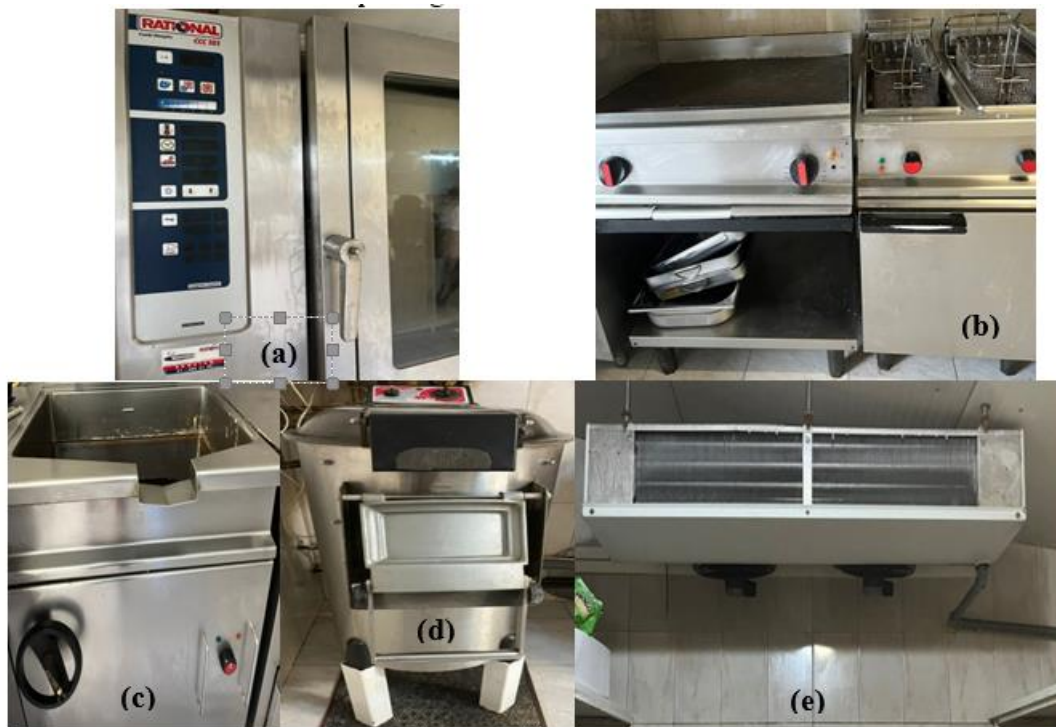
Figure 1. Pictures of kitchen equipment: (a) oven, (b) hob and fryer, (c) tilting pan, (d) potato peeler, (e) refrigerator
