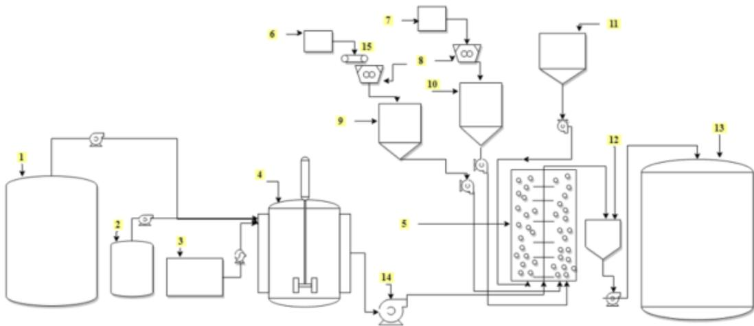
Figure 2. Process flow diagram proposed for the flax seed oil oleogel based cocoa spreads: 1 – Oil tank; 2 – Lecithin tank; 3 – Waxes tank; 4 – Oleogel preparation; 5 – Ball mill; 6 – Hazelnut storage; 7 – Sugar storage; 8 – Mill for sugar/hazelnut; 9 – Hazelnut paste tank; 10 – Powdered sugar; 12 – Cocoa; 13 – Cocoa spreadable cream; 14 – Circulating pumps; 15 – Conveyor belt
