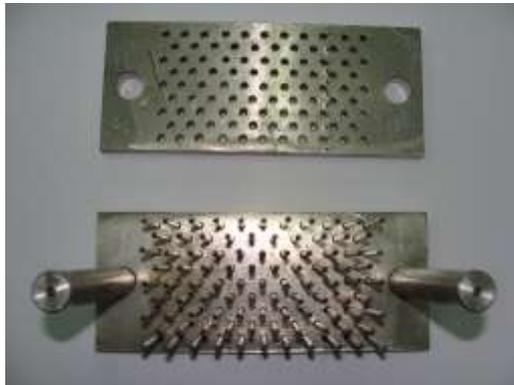
Figure 1. Multi - needle compression and piercing device
