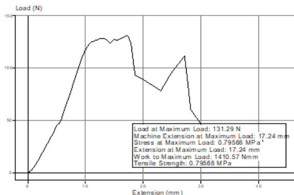
**Figure 7.** Warner - Bratzler shear force test diagram for “Pulpa Hituita” made by using 2500 N compression force (CP 2500.CVP)
