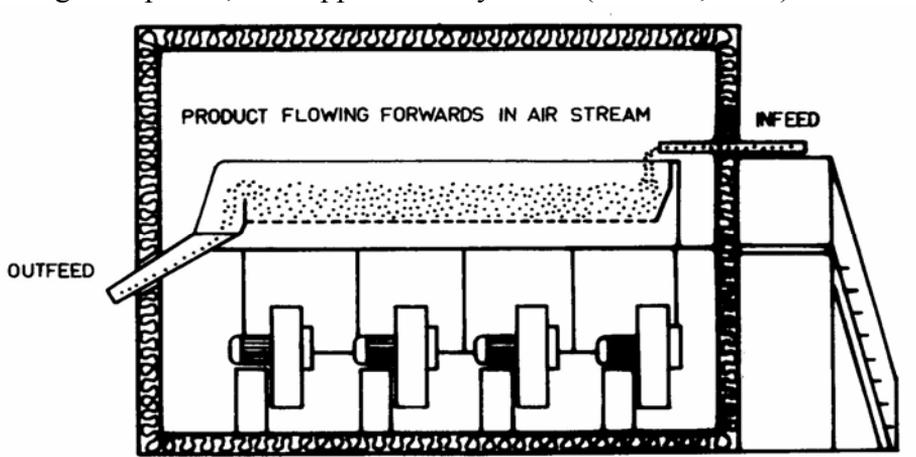
**Fig. 1.** – The freezing installation in fluidized bed of granular perishable products
