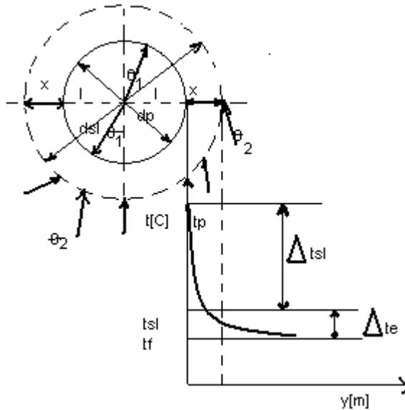
**Fig. 4.** – The temperature variation during the thermal transfer from the solid particle to the fluidization agent (Chiriac, 1982) ( $\Delta t_{sl}$  – the variation of temperature in the layer-limit;  $\Delta t_e$  – the variation of temperature in fluid;  $t_p$  – the temperature of solid particle;  $t_f$  – fluid temperature;  $d_{sl}$  – the diameter of layer-limit)
