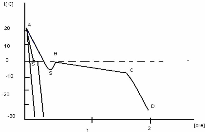
**Fig. 2.** – The variation of the product temperature during the freezing in fluidized bed (Tofan, 2002)
