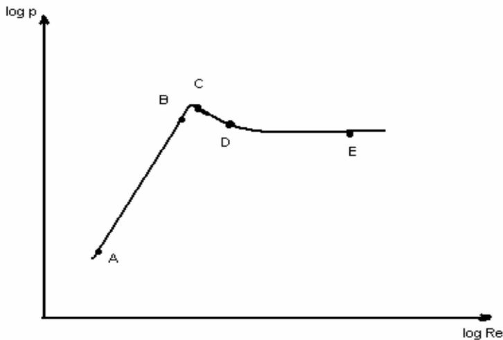
**Fig. 3.** – The variation of the pressure drop with the Reynolds number, at the flow through a granular bed (Tofan, 2002)
