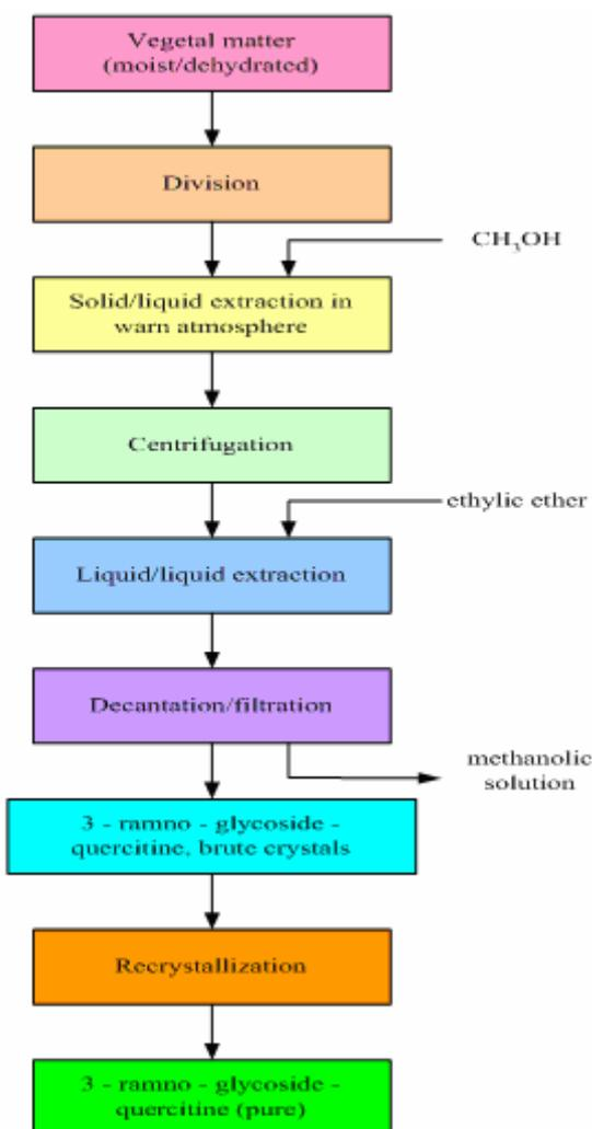
**Figure 1** Operation block scheme in the solid/liquid extraction process (methanol/ethyl ether operation variant) of 3 – ramno – glycoside quercitine from dog rose (*Rosa canina*)
