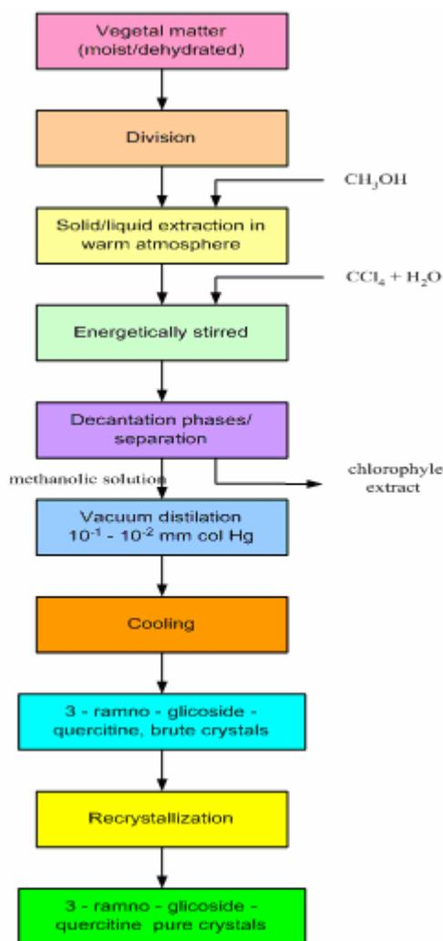
**Figure 2** Operation block scheme in the solid/liquid extraction process (methanol/carbon tetrachloride operation variant) of 3 – ramno – glycoside quercitine from dog rose (*Rosa canina*)
