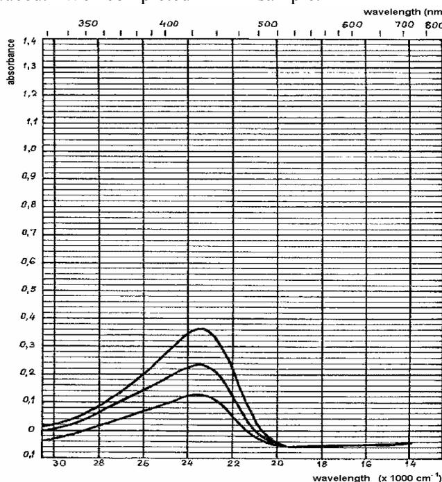
Figure 3 UV – VIS adsorption scheme of the solutions of different concentrations of 3 – ramno – glycoside quercitine
