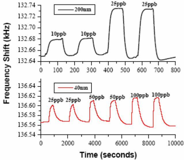
**Fig. 3.** InOx sensor responses towards ozone at optimal temperatures of 175°C and 230°C
