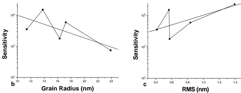
**Fig. 4.** The film sensitivity vs a) mean grain radius; b) surface roughness
