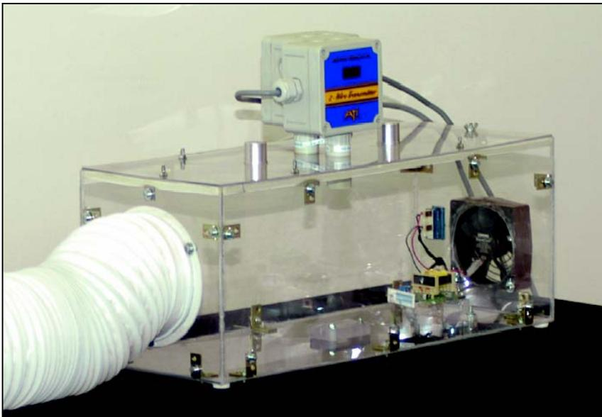
**Fig. 1.** Testing chamber with fan a PATT module and two sensors
