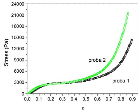
Figure 4. Compressive curve for bread with 30% whey sample
