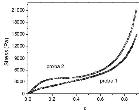
**Figure 2.** Compressive curve for bread control sample
