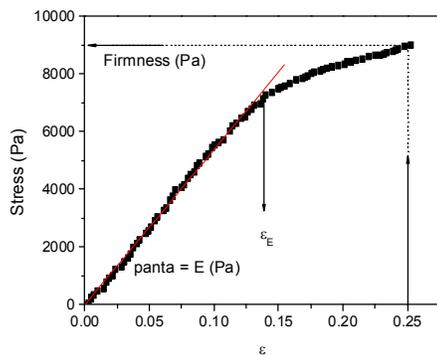
**Figure 1.** Dependence between compressive stress-strain
